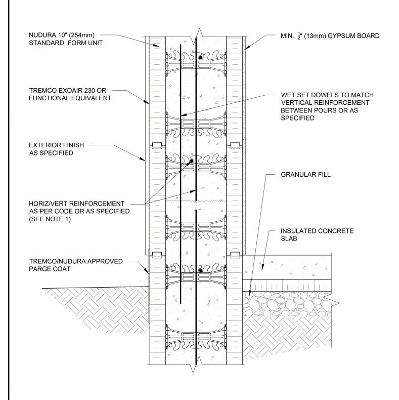
1) FOR OPTIMAL REINFORCEMENT PLACEMENT IN THE NUDURA FORM, SPACING OF HORIZONTAL REINFORCEMENT TO BE SPECIFIED AT 18" (457mm) O.C. AND VERTICAL REINFORCEMENT TO BE SPECIFIED AT MULTIPLES OF 8" (203mm) O.C. REFER TO NUDURA REINFORCEMENT PLACEMENT DETAILS.
