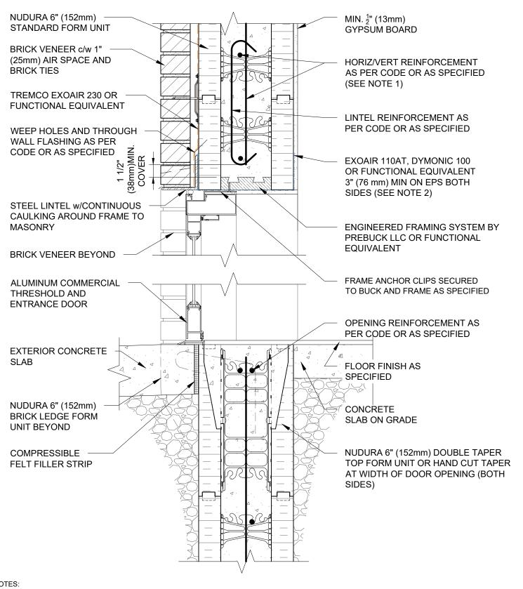
1) FOR OPTIMAL REINFORCEMENT PLACEMENT IN THE NUDURA FORM, SPACING OF HORIZONTAL REINFORCEMENT TO BE SPECIFIED AT 18" (457mm) O.C. AND VERTICAL REINFORCEMENT TO BE SPECIFIED AT MULTIPLES OF 8" (203mm) O.C. REFER TO NUDURA REINFORCEMENT PLACEMENT DETAILS. 2) AIR BARRIER/DRAINAGE FLASHINGS TO BE INSTALLED AROUND COMPLETE OPENING PERIMETER AS PER TREMCO/NUDURA APPLICATION INSTRUCTIONS OR AS DETAILED BY LOCAL APPLICABLE CODES (CODE GOVERNS).
