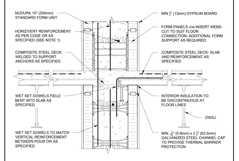
1) FOR OPTIMAL REINFORCEMENT PLACEMENT IN THE NUDURA FORM, SPACING OF HORIZONTAL REINFORCEMENT TO BE SPECIFIED AT 18" (457mm) O.C. AND VERTICAL REINFORCEMENT TO BE SPECIFIED AT MULTIPLES OF 8" (203mm) O.C. REFER TO NUDURA REINFORCEMENT PLACEMENT DETAILS.
