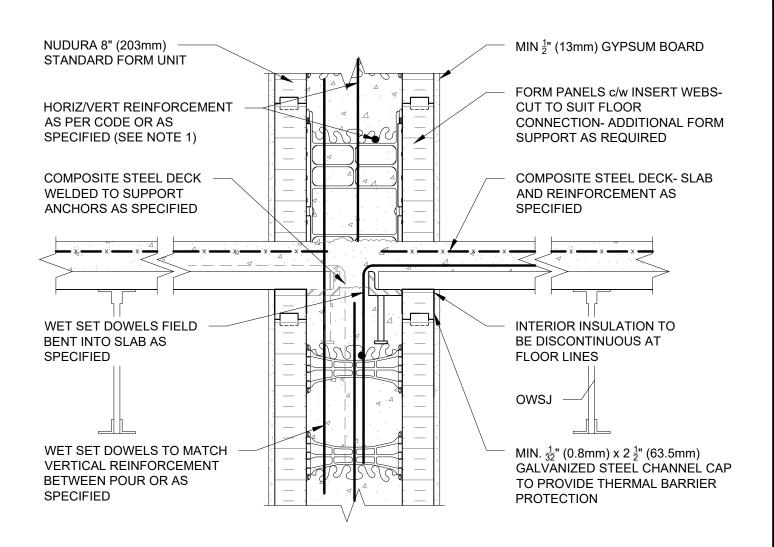
1) FOR OPTIMAL REINFORCEMENT PLACEMENT IN THE NUDURA FORM, SPACING OF HORIZONTAL REINFORCEMENT TO BE SPECIFIED AT 18" (457mm) O.C. AND VERTICAL REINFORCEMENT TO BE SPECIFIED AT MULTIPLES OF 8" (203mm) O.C. REFER TO NUDURA REINFORCEMENT PLACEMENT DETAILS.
