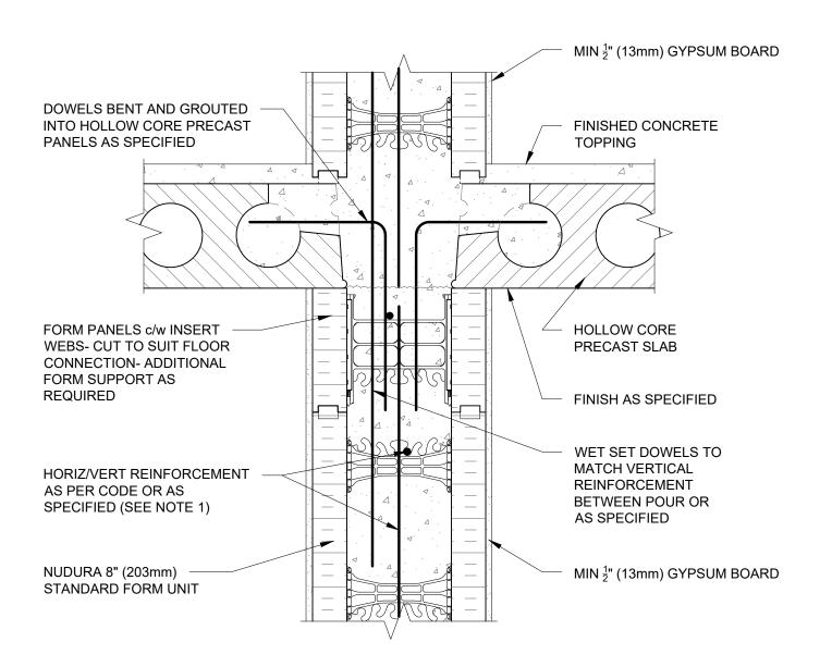
1) FOR OPTIMAL REINFORCEMENT PLACEMENT IN THE NUDURA FORM, SPACING OF HORIZONTAL REINFORCEMENT TO BE SPECIFIED AT 18" (457mm) O.C. AND VERTICAL REINFORCEMENT TO BE SPECIFIED AT MULTIPLES OF 8" (203mm) O.C. REFER TO NUDURA REINFORCEMENT PLACEMENT DETAILS.
