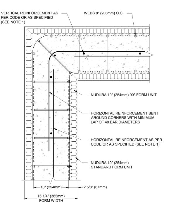
1) FOR OPTIMAL REINFORCEMENT PLACEMENT IN THE NUDURA FORM, SPACING OF HORIZONTAL REINFORCEMENT TO BE SPECIFIED AT 18" (457mm) O.C. AND VERTICAL REINFORCEMENT TO BE SPECIFIED AT MULTIPLES OF 8" (203mm) O.C. REFER TO NUDURA REINFORCEMENT PLACEMENT DETAILS.
