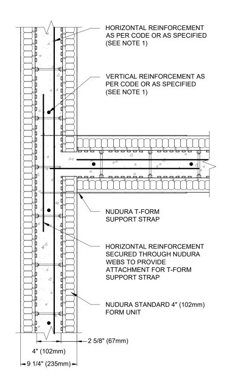
1) FOR OPTIMAL REINFORCEMENT PLACEMENT IN THE NUDURA FORM, SPACING OF HORIZONTAL REINFORCEMENT TO BE SPECIFIED AT 18" (457mm) O.C. AND VERTICAL REINFORCEMENT TO BE SPECIFIED AT MULTIPLES OF 8" (203mm) O.C. REFER TO NUDURA REINFORCEMENT PLACEMENT DETAILS.
