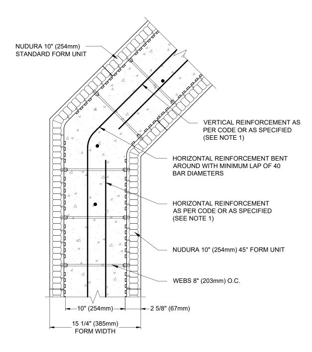
1) FOR OPTIMAL REINFORCEMENT PLACEMENT IN THE NUDURA FORM, SPACING OF HORIZONTAL REINFORCEMENT TO BE SPECIFIED AT 18" (457mm) O.C. AND VERTICAL REINFORCEMENT TO BE SPECIFIED AT MULTIPLES OF 8" (203mm) O.C. REFER TO NUDURA REINFORCEMENT PLACEMENT DETAILS.
