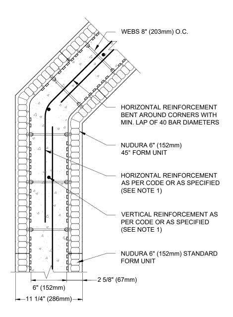
1) FOR OPTIMAL REINFORCEMENT PLACEMENT IN THE NUDURA FORM, SPACING OF HORIZONTAL REINFORCEMENT TO BE SPECIFIED AT 18" (457mm) O.C. AND VERTICAL REINFORCEMENT TO BE SPECIFIED AT MULTIPLES OF 8" (203mm) O.C. REFER TO NUDURA REINFORCEMENT PLACEMENT DETAILS.
