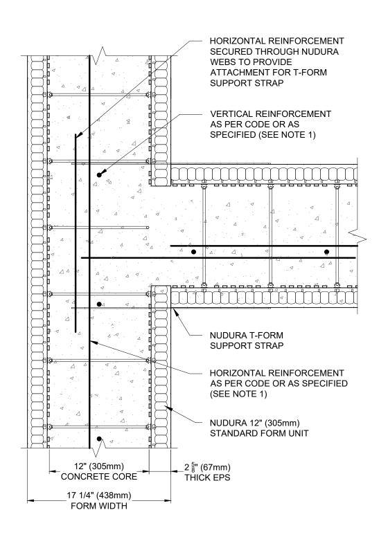
1) FOR OPTIMAL REINFORCEMENT PLACEMENT IN THE NUDURA FORM, SPACING OF HORIZONTAL REINFORCEMENT TO BE SPECIFIED AT 18" (457mm) O.C. AND VERTICAL REINFORCEMENT TO BE SPECIFIED AT MULTIPLES OF 8" (203mm) O.C. REFER TO NUDURA REINFORCEMENT PLACEMENT DETAILS.
