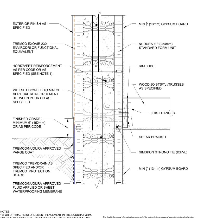
FOR OPTIMAL REINFORCEMENT PLACEMENT IN THE NUDURA FORM, SPACING OF HORIZONTAL REINFORCEMENT TO BE SPECIFIED AT 18" (457mm) O.C. AND VERTICAL REINFORCEMENT TO BE SPECIFIED AT MULTIPLES OF 8" (203mm) O.C. REFER TO NUDURA REINFORCEMENT PLACEMENT DETAILS.
