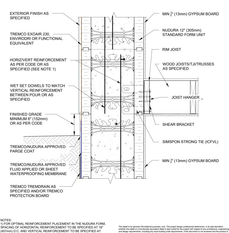
SPACING OF HORIZONTAL REINFORCEMENT TO BE SPECIFIED AT 18" (457mm) O.C. AND VERTICAL REINFORCEMENT TO BE SPECIFIED AT MULTIPLES OF 8" (203mm) O.C. REFER TO NUDURA REINFORCEMENT PLACEMENT DETAILS.
