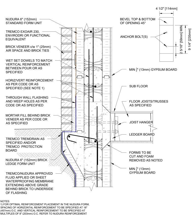
PLACEMENT DETAILS. 2.2) THIS DETAIL IS TO BE USED ONLY AS AN EXAMPLE OF THE POTENTIAL GRADE LEVEL ALLOWED IN SPECIFIC GEOGRAPHICAL LOCATIONS. GRADE LEVEL TO BE VERIFIED BY LOCAL BUILDING
