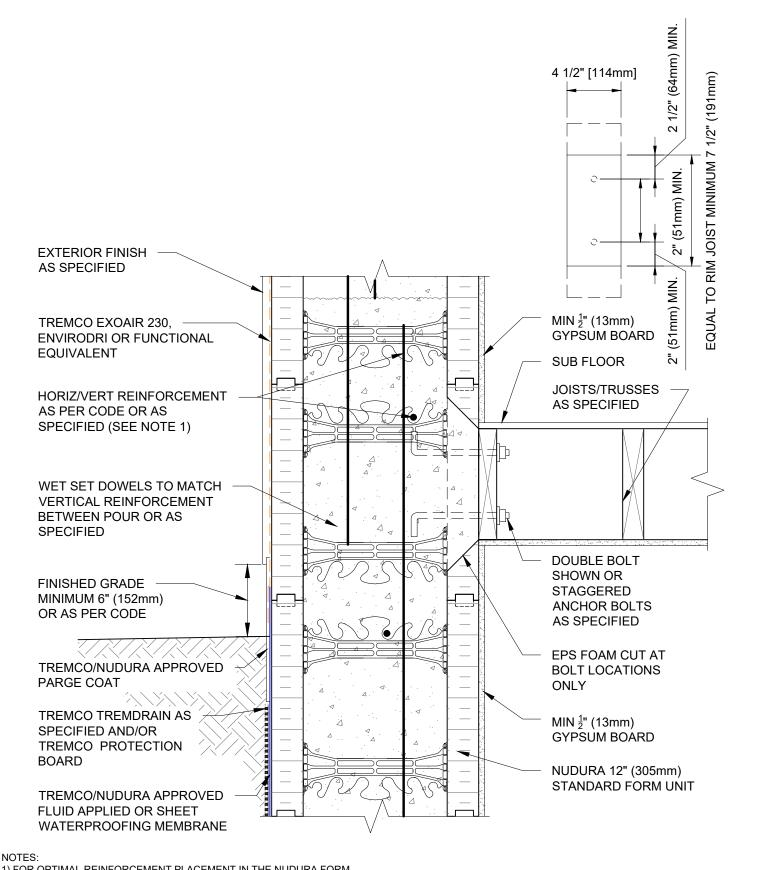
1) FOR OPTIMAL REINFORCEMENT PLACEMENT IN THE NUDURA FORM, SPACING OF HORIZONTAL REINFORCEMENT TO BE SPECIFIED AT 18" (457mm) O.C. AND VERTICAL REINFORCEMENT TO BE SPECIFIED AT MULTIPLES OF 8" (203mm) O.C. REFER TO NUDURA REINFORCEMENT PLACEMENT DETAILS.
