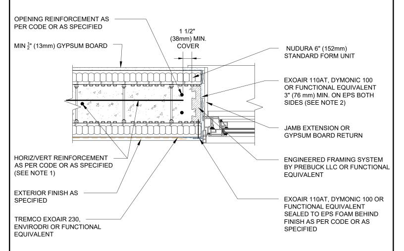
1) FOR OPTIMAL REINFORCEMENT PLACEMENT IN THE NUDURA FORM, SPACING OF HORIZONTAL REINFORCEMENT TO BE SPECIFIED AT 18" (457mm) O.C. AND VERTICAL REINFORCEMENT TO BE SPECIFIED AT MULTIPLES OF 8" (203mm) O.C. REFER TO NUDURA REINFORCEMENT PLACEMENT DETAILS.
