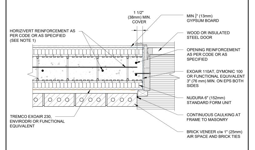
1) FOR OPTIMAL REINFORCEMENT PLACEMENT IN THE NUDURA FORM, SPACING OF HORIZONTAL REINFORCEMENT TO BE SPECIFIED AT 18" (457mm) O.C. AND VERTICAL REINFORCEMENT TO BE SPECIFIED AT MULTIPLES OF 8" (203mm) O.C. REFER TO NUDURA REINFORCEMENT PLACEMENT DETAILS.
