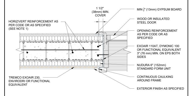
1) FOR OPTIMAL REINFORCEMENT PLACEMENT IN THE NUDURA FORM, SPACING OF HORIZONTAL REINFORCEMENT TO BE SPECIFIED AT 18" (457mm) O.C. AND VERTICAL REINFORCEMENT TO BE SPECIFIED AT MULTIPLES OF 8" (203mm) O.C. REFER TO NUDURA REINFORCEMENT PLACEMENT DETAILS.
