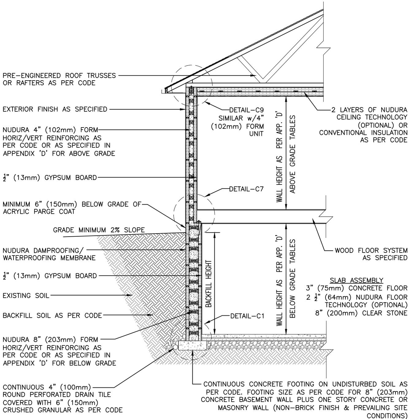
\*NOTE: IN ADDITION TO FOOTING SIZE INDICATED BY CODE, ADD 1" (25.4mm) WIDTH TO STRIP FOOTING FOR EVERY 1'0" (305mm) OF CONCRETE WALL HEIGHT ABOVE 8'0" (2440m) PER STORY
